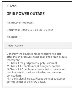
figure 7-9 Detailed Fault Alarm Information
