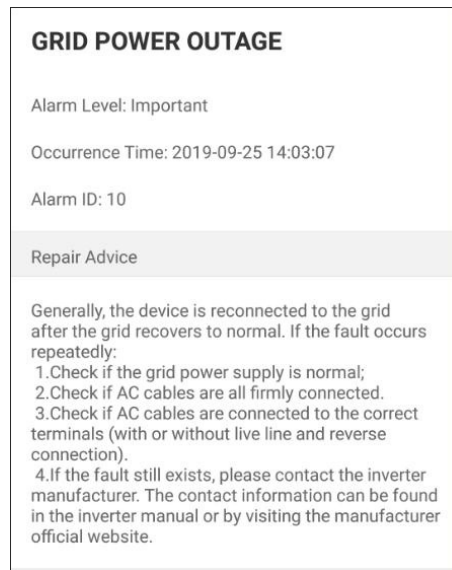
figure 7-9 Detailed fault alarm info
